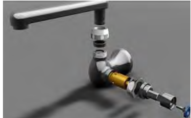
Exploded view of new taps installed in the handwash areas; an interactive visual aid for maintenance purposes.
